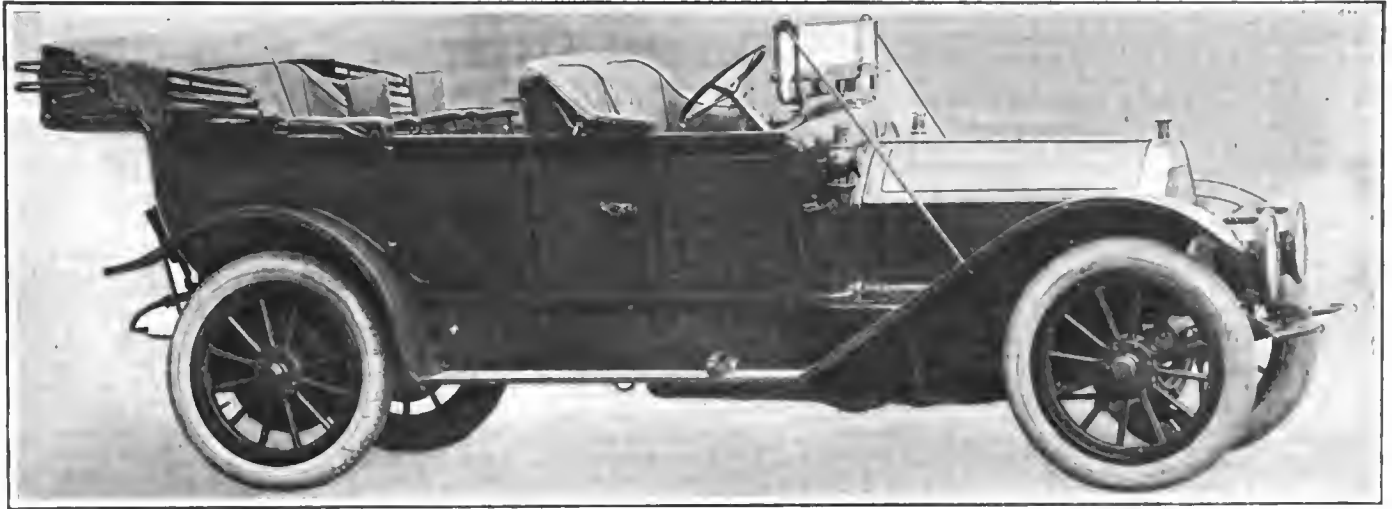
Fig. 4—48-horsepower seven-passenger touring car with fore-door flush-sided body
